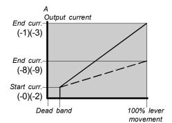
\* The speed reduction function reduces proportionally maximum available output current, between the values of parameter (-1)/(-3) and (-8)/(-9), as the vehicle groundspeed changes between a speed corresponding to value of parameter (-6) and (-7). This enabling the sensitivity of the steering to decrease as the vehicle speed increase.
