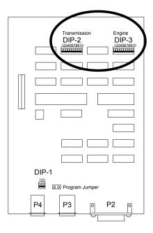
The switch marked DIP-2 adjusts the transmission input, and DIP-3 the engine input. To adjust the switches a small instrument of some kind is needed, a pencil is usually Adequate.
